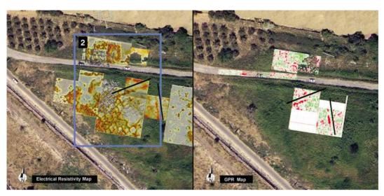
Fig. 4. Maps of electrical resistivity (left) and GPR surveys (right) showing the main linear feature in Areas A and B.
